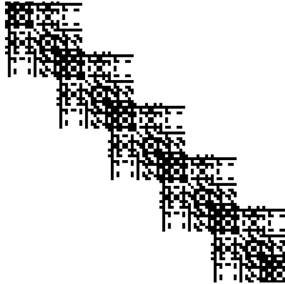
Figure 6: Non-zero entries of the stiffness matrix for the mesh shown in Fig. 4 with ten-node quadratic tetrahedral elements.
